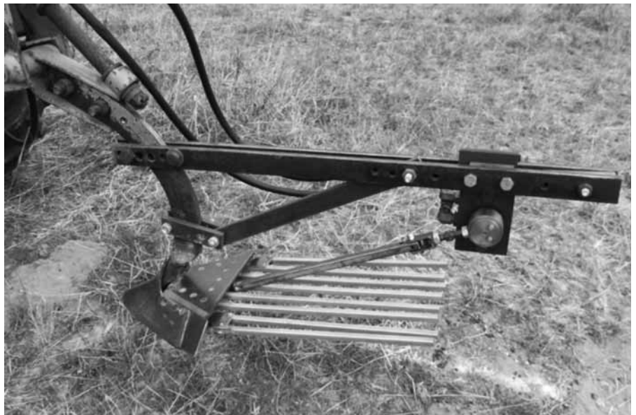
Experimental rig to evaluate digging and sieving of anti-personnel mines
